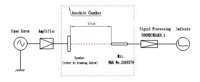
The speaker, being tested in an anechoic chamber, is installed in a baffle of 135cmx165cm.
